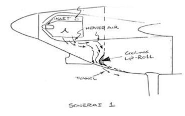
screwed to the bottom corner of the firewall, to keep hot air flow attached to change direction as it exits thru the tunnel.
